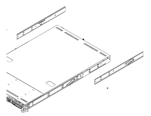
Figure 2-2. Installing the Rack Rails
